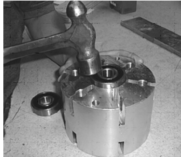
Figure 77. Tap outer race of new bearing, alternating sides
